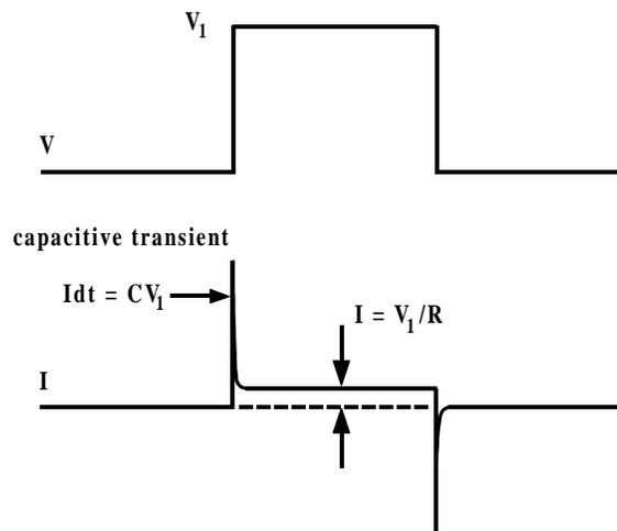
**Figure 1-15.** Typical Voltage-Clamp Experiment
