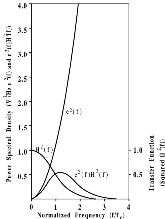
**Figure 12-6.** Squared Transfer Function of a Gaussian Filter
