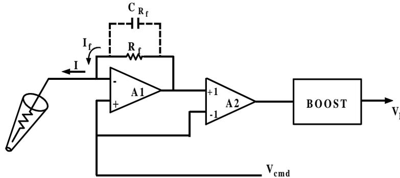
**Figure 3-22.** Resistive Headstage
