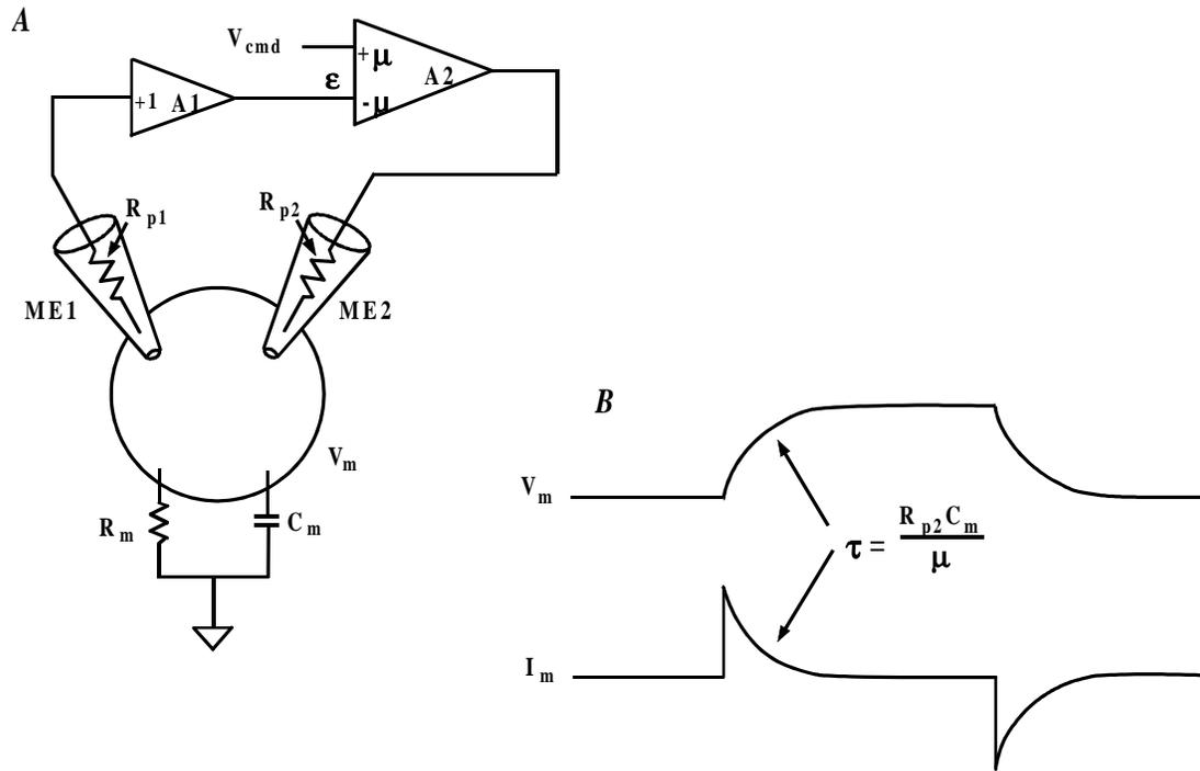
**Figure 3-12.** Conventional Two-Electrode Voltage Clamp
