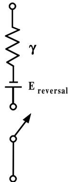
**Figure 1-4.** Equivalent Circuit for a Single-Membrane Channel
