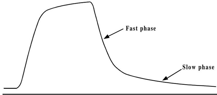
**Figure 3-14.** Biphasic Voltage Response of a High-Resistance Micropipette
