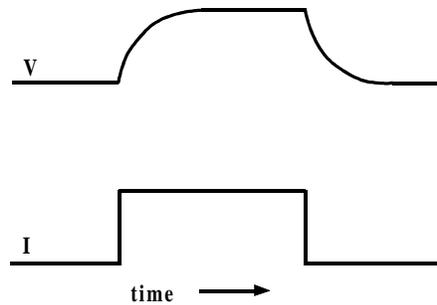
**Figure 1-14.** RC Parallel Circuit Response
