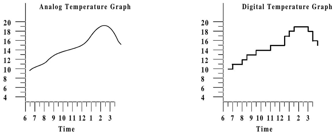
**Figure 9-1.** Analog-to-Digital Conversion
