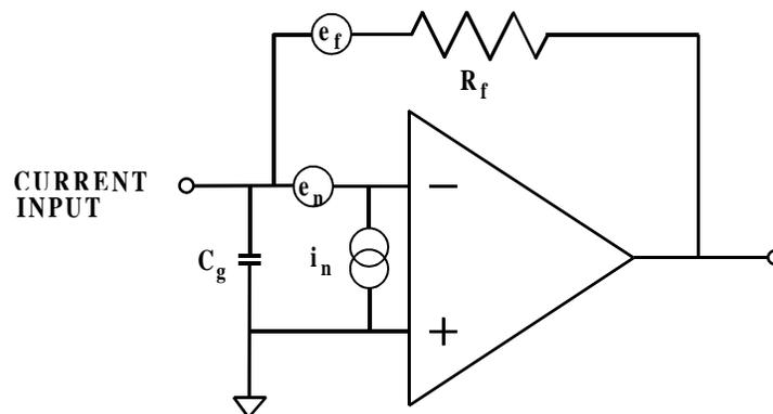
Figure 12-3. Noise Model of a Simplifier Current-to-Voltage Converter
