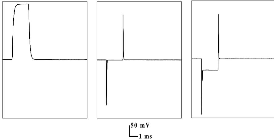
**Figure 3-5.** Illustration of Bridge Balancing While Micropipette is Extracellular
