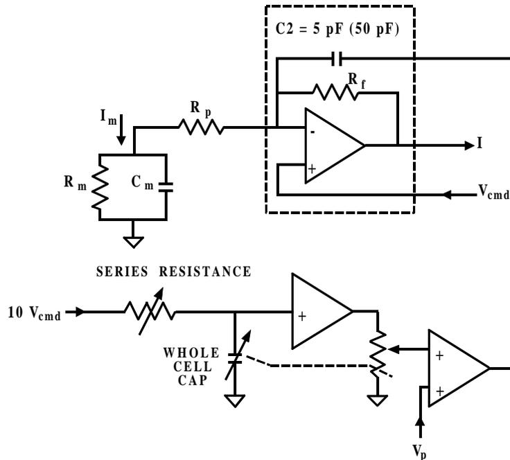
**Figure 3-20.** Whole-Cell Capacitance Compensation Circuit
