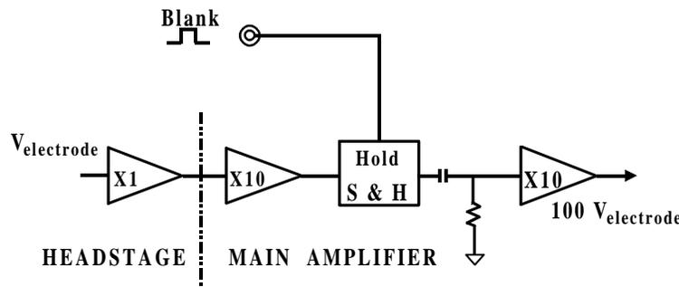
**Figure 3-1.** Blanking Circuit
