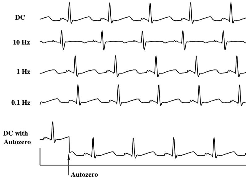
**Figure 6-8.** Comparison of Autozeroing to AC Coupling
