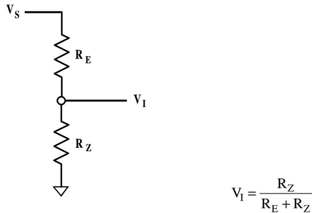
**Figure 7-2.** High Electrode Resistance Can Attenuate a Signal and Increase Crosstalk
