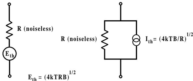
**Figure 12-1.** Noise Equivalent Circuits of a Resistor
